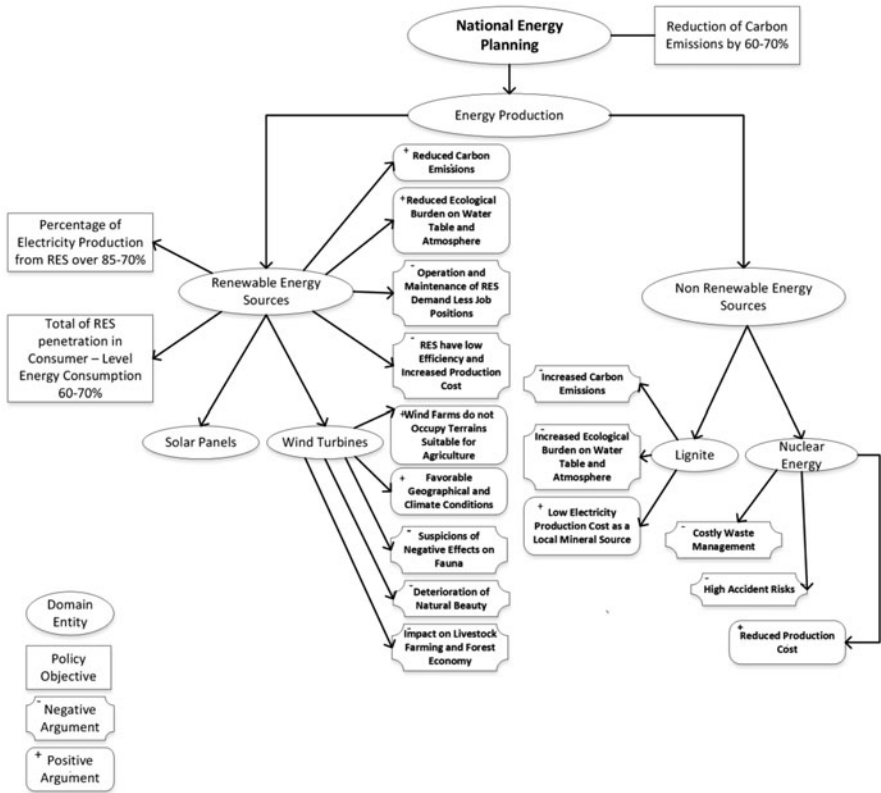
Fig. 12.7 Energy policy model based on the above energy domain model (including policy statements and arguments)
